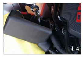
Using both thumbs, push the ears of the clamp outwards to fully tighten clamp. See ill. 5
