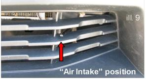
**Operation-** Slide the adjustable lever horizontally to the desired position. The "air intake" position blocks the brake duct and directs virtually all of the incoming air to the air box area. The "brake duct" position directs the majority of the air to the brake duct portion while still supplying some additional air to the intake. This is possible because the Big Gulp has a larger entry which uses the entire available opening.
