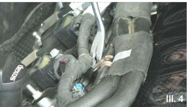
Locate the #1 left engine cover, (2) of the #4 lower grommets and (2) of the #5 upper "horseshoe" grommets. Install the lower round grommets by pushing into the mounting tubes on the engine cover, then turning appr. 1/2 turn to fully seat. Install the upper "horseshoe" grommets by hooking one side over on of the tangs on the upper brackets then pushing the other side over the remaining tang. Repeat this process for the #2 right engine cover and the remaining grommets.
