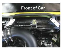
Repeat the bracket installation procedure for the right side remembering to apply inward pressure during final tighening. Be careful not to over tighten! See Fig. 3 for reference.
