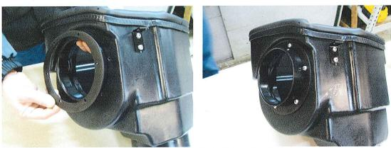
Step 8. Locate #3 "L" bracket. Install "L" bracket to Roto-Fab air box. Using the supplied 10-32 SS machine screws, fasten the bracket to the front side of the Roto-Fab air box. \*Note: Install the head of the machine screws from the outside of the air box.
