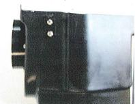
Step 9. Locate #14 Coolant Reservoir Bracket. Install the Coolant Reservoir Bracket. Using the supplied 10-32 SS machine screws, fasten the bracket to the back side of the Roto-Fab air box. \*Note: Install the head of the machine screws from the inside of the air box.
