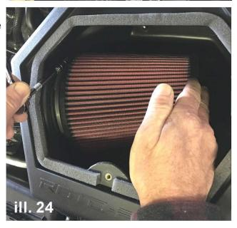
Close the air box lid and look under the lid to align the screw with the threaded brass insert on the air box. With the screw properly aligned, tighten the screw down to the point that the lid is approximately flush with the top side of the air box.
