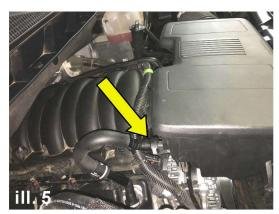
NOTE: During the next steps you will not disconnect the wiring harness from the MAF sensor. It will remain plugged in through the entire dissassembly and assembly process.
