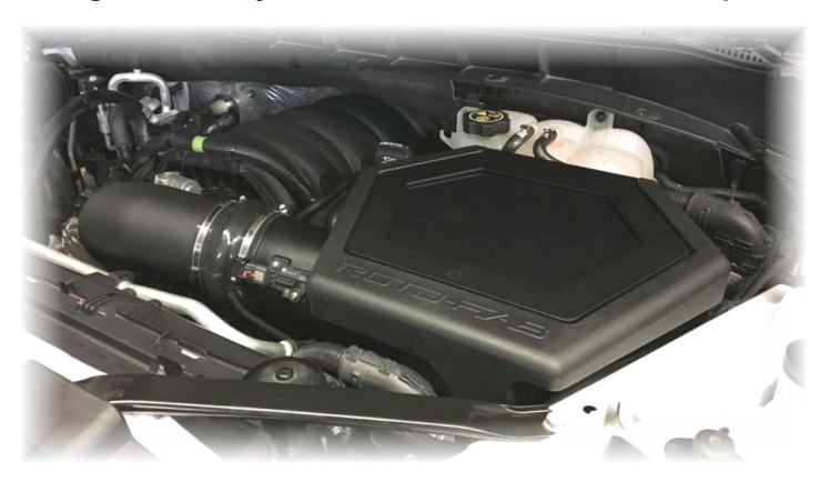
All clamps should be checked for tightness after a few drive cycles and periodically thereafter. Inspect hose clamps for tightness at each oil change. Inspect the filter approximately every third oil change - more often in dusty regions. Service the filter as necessary using the proper service kit. Filter service kits are available at roto-fab.com
