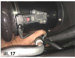
Standing in front of the vehicle, use your left hand to reach under the MAF sensor housing to engage the gray loom holer into the 1/4 " hole on air box just below MAF housing. Push firmly to engage as much as possible. See ill. 17
