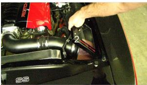
Install the stock stiffener brace which was previously removed. Double check to be sure the MAF sensor is plugged in, the breather hose is properly connected and the hose clamps are tight. Your installation is now complete!
