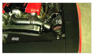
Locate the #2 air box lid assembly. Angle the lid so the water deflector portion goes completely *under* the lip of the fender. Next, align the 1/2 turn fasteners with the inserts on the air box. With all four fasteners aligned, use a philips screwdriver to engage all four fasteners.
