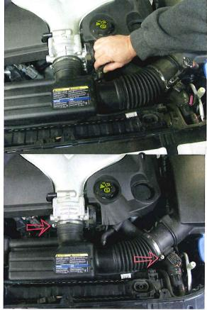
Step 2. Disconnect MAF sensor connector. Using your fingers, squeeze and pull firmly to disconnect the MAF sensor harness and remove MAF sensor.
