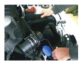
Step 4. Place the windshield washer fluid neck back to its original location and hand tighten the mounting bolt. Do not tighten this bolt at this time.
