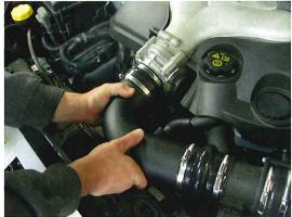
Step 13. Align and tighten the hose clamp that secures the 4" hump hose to the air inlet elbow. At this time, Double check all of the installed hose clamps for tightness.
