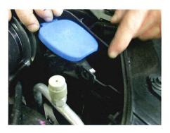
Step 7. IMPORTANT. Adjust airbox assembly to its full counter clockwise position and hold in place while tightening mounting bolt and nut. The airbox should be in contact with the windshield washer fluid cap.
