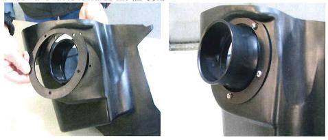
\* Note: Align notch in flange with the guide on the filter housing. This image shows the raw flange better show the details.
