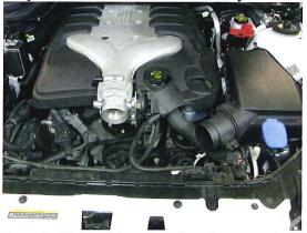
Step 4. Using 10mm socket. Remove 10mm nuts from air box assembly.
