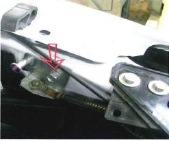
Step 8. Using T25 torx bit. Remove 2 bolts holding the MAF sensor to factory air box. Remove MAF sensor from factory air box assembly.
