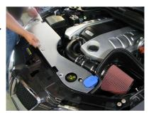
Step 3. Insert the four push fasteners to secure the cover. if the lip of the cover is not hooked under one of the protrusions on the W/W fill tube. Adjust if necessary.
